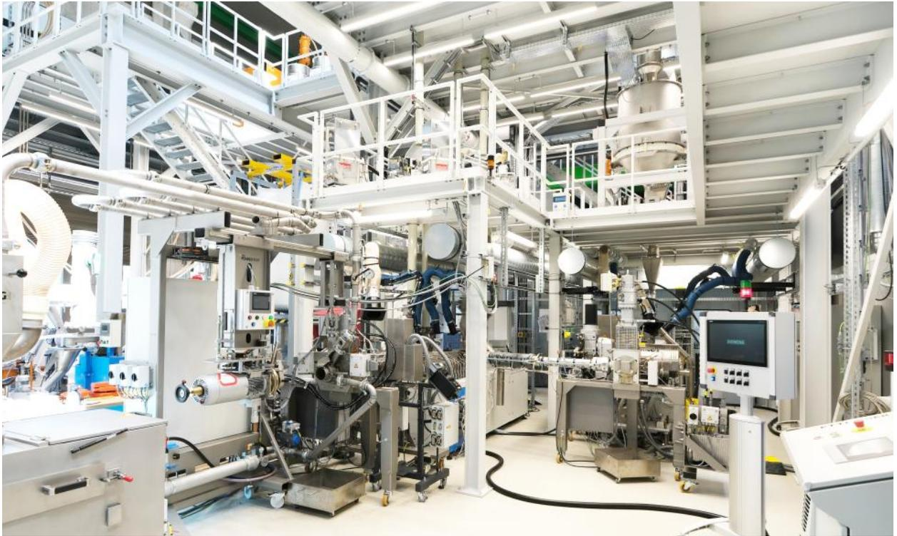
*EdelWeissCompounding Technology - Multivariable adaptive Tandem-Extruderlinie. Foto: IKK*
