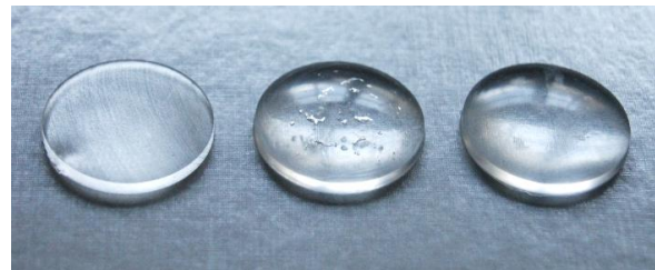
Preliminary tests for the production of highly transparent silicone lenses
