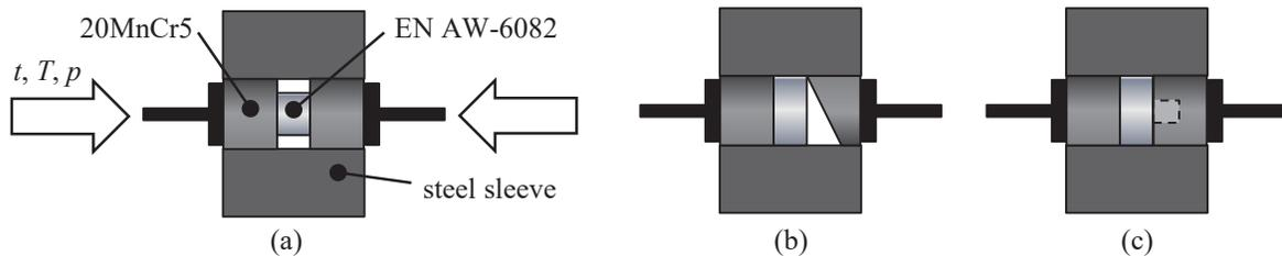
FIGURE 3. Schematic of dilatometer tests using different steel specimens, (a) cylindrical, (b) chamfered, (c) bored
