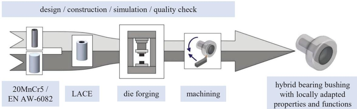
**FIGURE 1.** Novel process chain to manufacture a hybrid bearing bushing consisting of aluminium and steel, starting with a LACE process, followed by subsequent die forging and machining processes [2]
