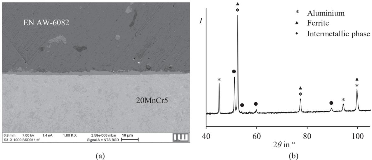
**FIGURE 6.** Aluminium (EN AW-6082) and steel (20MnCr5) dilatometer specimen compressed for 240 s at 540 °C with 5890 N; (a) BSD image of the interface; (b) XRD pattern of the interface with main peaks for aluminium and steel and additional peaks from an intermetallic phase
