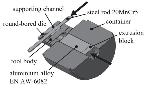
FIGURE 2. Schematic sectional view of the LACE process with a redirection of the aluminium alloy by an angle of 90°
