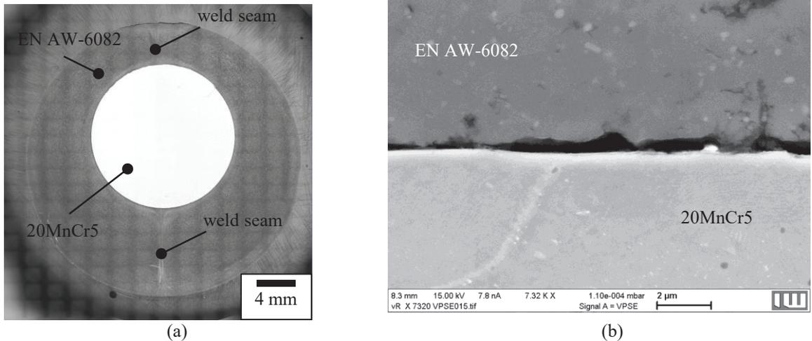
**FIGURE 5.** (a) Light optical image of the cross section after a profile length of 75 mm; (b) SEM image of the interface between EN AW-6082 and 20MnCr5 after an aluminium length of 390 mm
