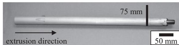
**FIGURE 4.** Co-extruded aluminium steel profile with a total diameter of 28 mm and a total aluminium length of 540 mm
