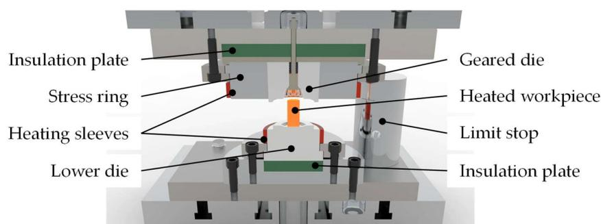
**Figure 3.** Forging tool system for manufacturing hybrid bevel gears.
