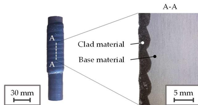
**Figure 2.** Material distribution in plasma transferred arc (PTA) cladded workpiece for a 41Cr4/C22.8 combination with an initial substrate diameter of  $\varnothing$  27 mm along the cutting line A-A (longitudinal cross section).
