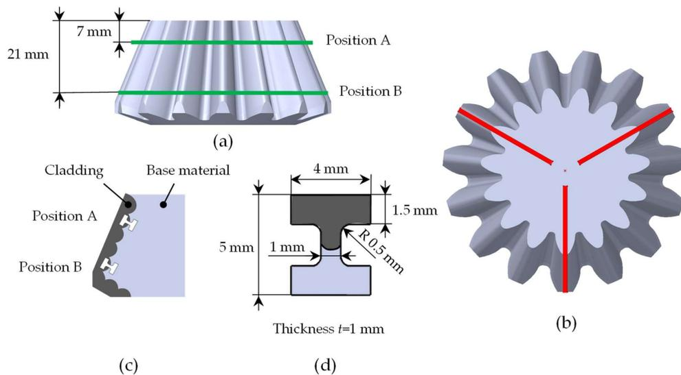
**Figure 7.** Sampling positions of the cross-sectional micrographs for metallographic examination and hardness measurements (a), extraction position of the sample plates (b), extraction position of the tensile specimens from the sample plates (c), geometry of the micro tensile specimen (d).
