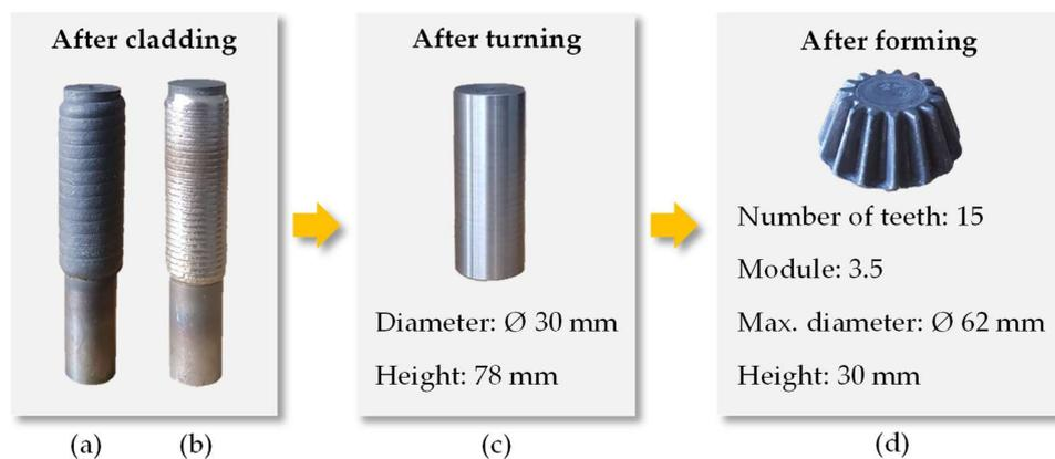
**Figure 1.** Cladded preforms produced with plasma transferred arc deposition welding (PTAW) (a) and laser hotwire cladding (LHC) (b) using a substrate with a diameter of 27 mm; geometry of the turned workpiece (c) and bevel gear (d).
