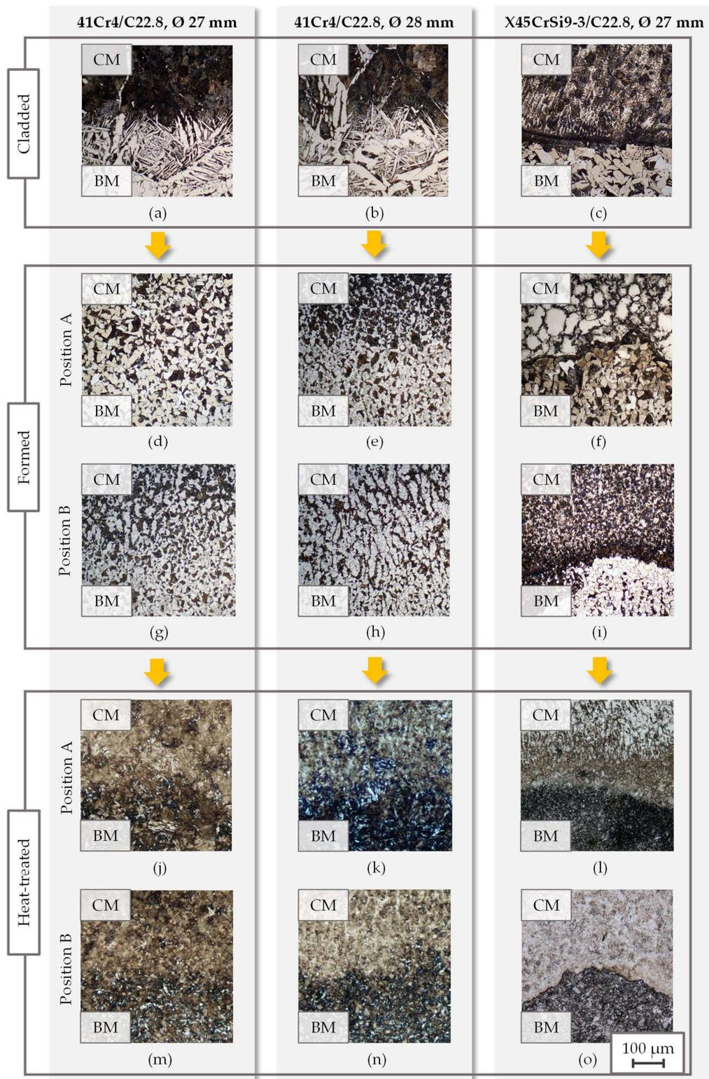
**Figure 8.** Microstructural evolution in the material combinations 41Cr4/C22.8 and X45CrSi9-3/C22.8 after cladding (a–c), forming (d–i) and heat-treatment (j–o); etched with 5% nitric acid solution excluding (c,f,i)—etched with Beraha II reagent—and (l,o)—Etched with V2A etchant.
