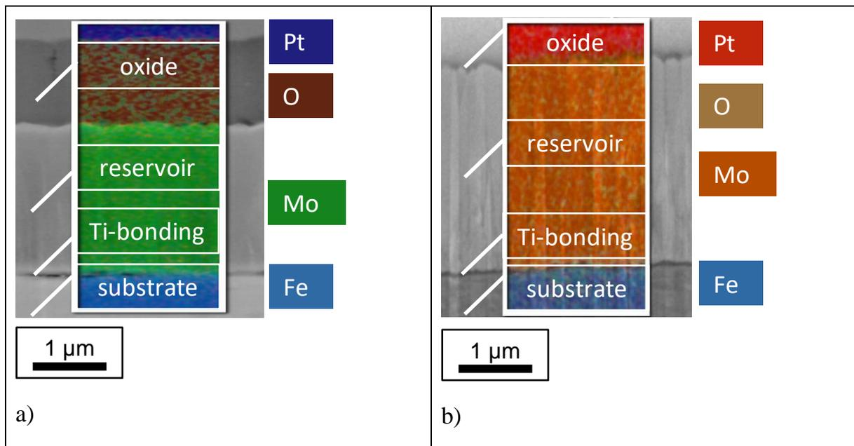
Figure 3: cross sections prepared using focussed ion beam 3a) Molybdenum oxide (sputtered with  $\text{MoO}_3$  target) 3b) Molybdenum oxide (sputtered reactively)
