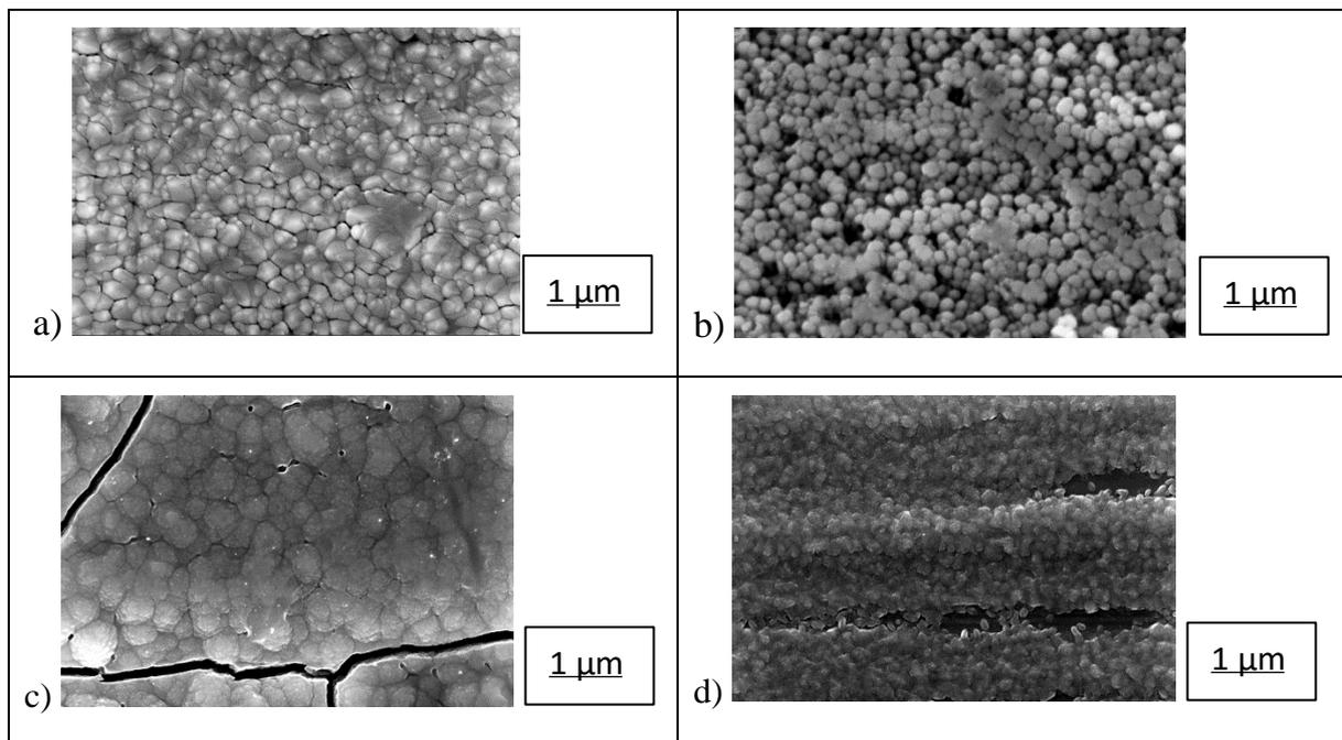
Figure 2: SE images of different sputter conditions 2a) pure Molybdenum 2b) Molybdenum oxide (sputtered reactively) 2c) Molybdenum oxide (sputtered with  $\text{MoO}_3$  target) 2d) pure Ti
